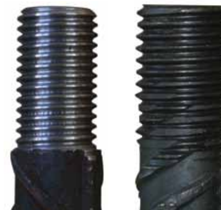
Threads on a non-upsetted rebar.
